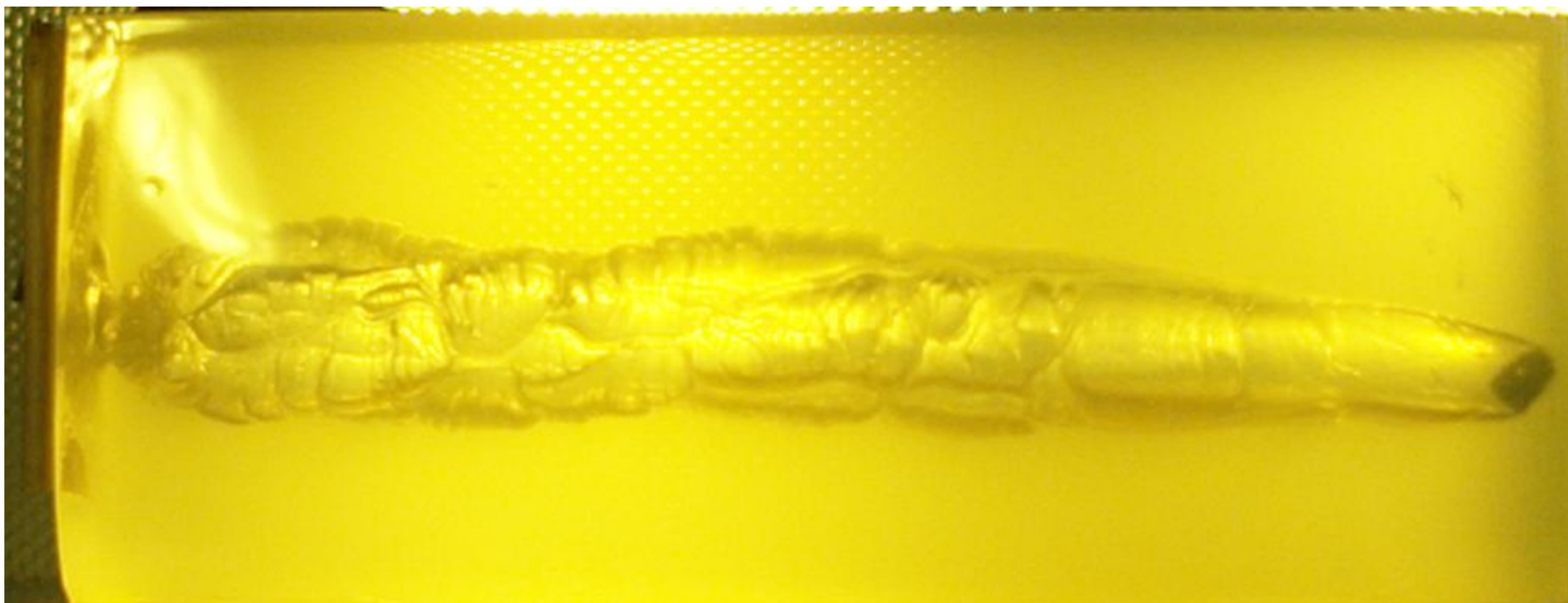
45 Auto Remington Golden Saber 230gr failure to expand after striking bone
