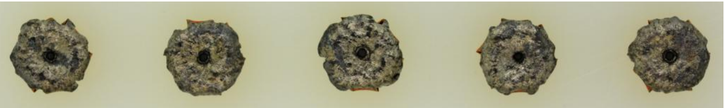
9mm Luger Hornady XTP 124gr through bare gelatin
