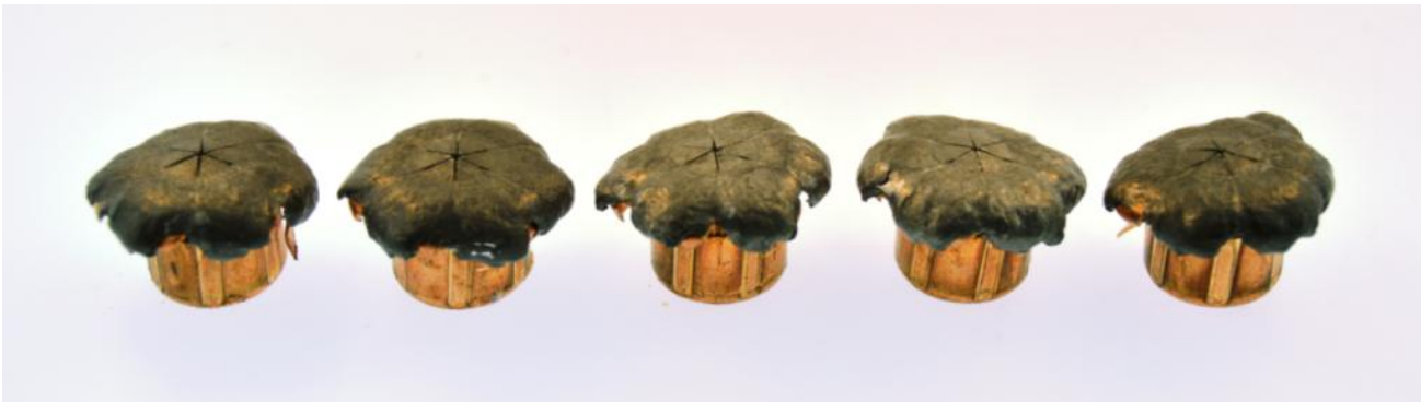
Bullets recovered from the FBI Heavy clothing setup
