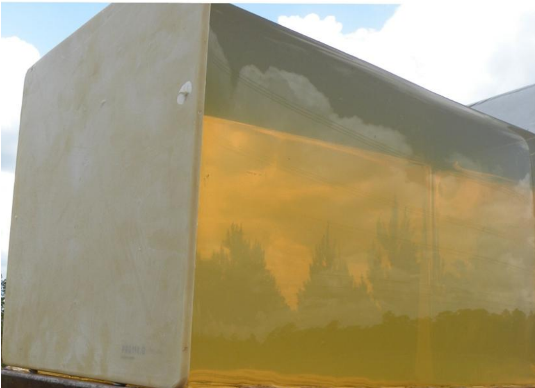
Synbone 6mm thick bone simulant plate in front of bare gelatin block
