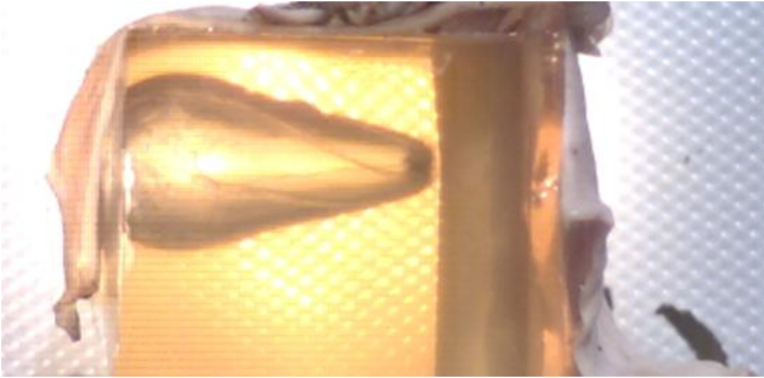
Femur simulant target (pig skin, 10% gelatin, bone tube, 10% gelatin, pig skin)
