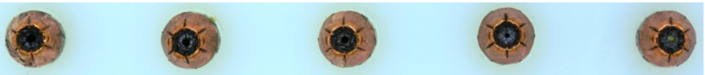
9mm Luger Hornady XTP 124gr through bone plate
