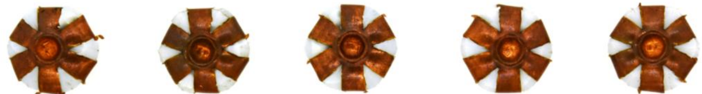
9mm Luger Federal EFMJ 105gr through bare gelatin
