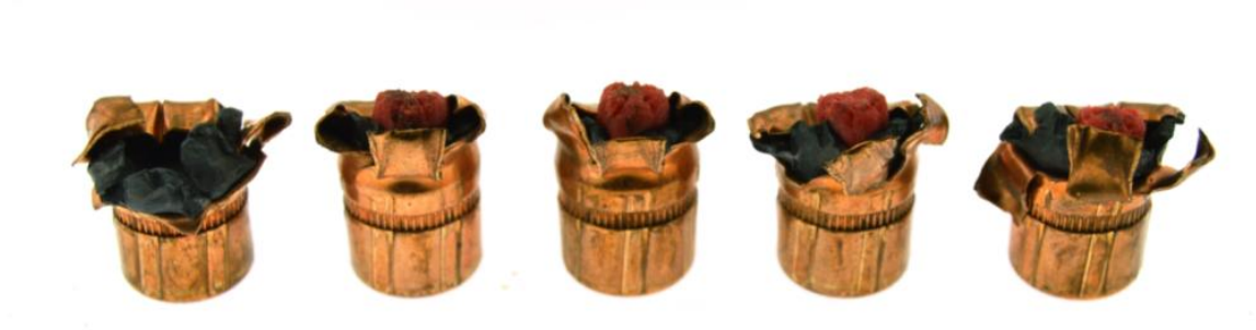
Bullets recovered from the FBI Wallboard setup
