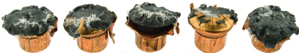
Bullets recovered from the FBI Steel setup
