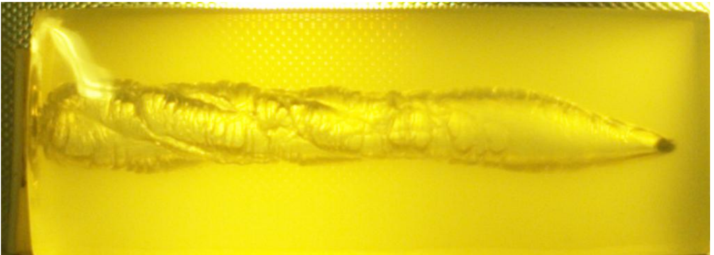
9mm Luger Remington Golden Saber 124gr failure to expand after striking bone
