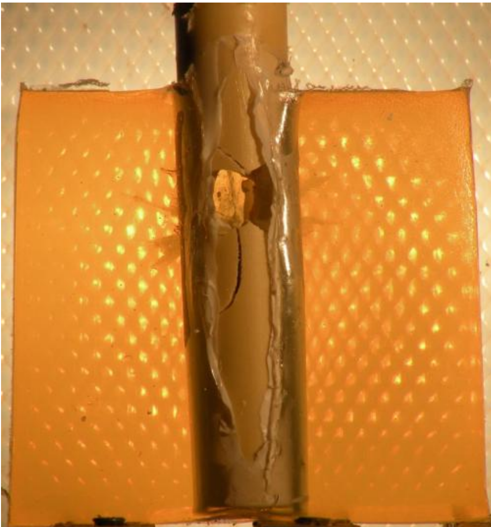
Rear view of femur simulant target shot by 9mm JHP. Note complete fracturing of bone.
