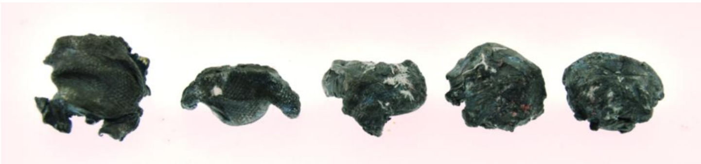
Bullets recovered from the FBI Auto Glass setup
