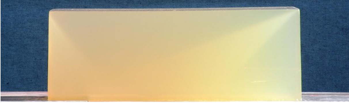
Bare gelatin (10% ballistic gelatin block)
