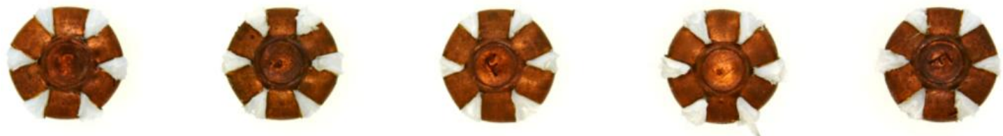
9mm Luger Federal EFMJ 105gr through bone plate
