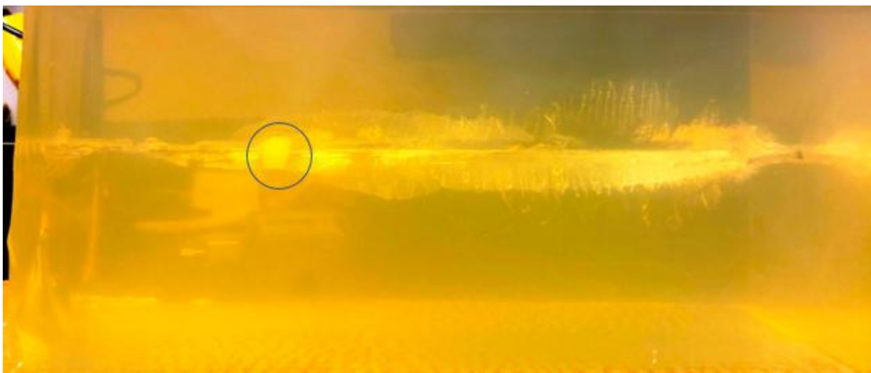
Sphere and rod being pulled through the gelatin wound track (sphere circled)
