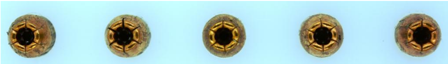
45 Auto +P Winchester Ranger-T 230gr through bone plate
