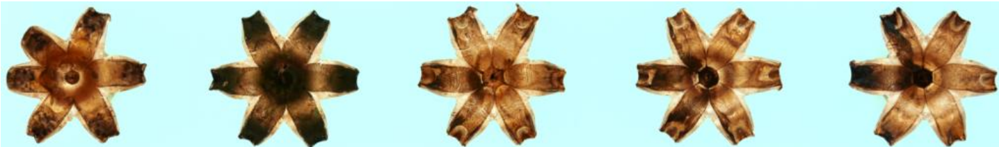
9mm Luger +P Cor-Bon DPX 115gr through bone plate
