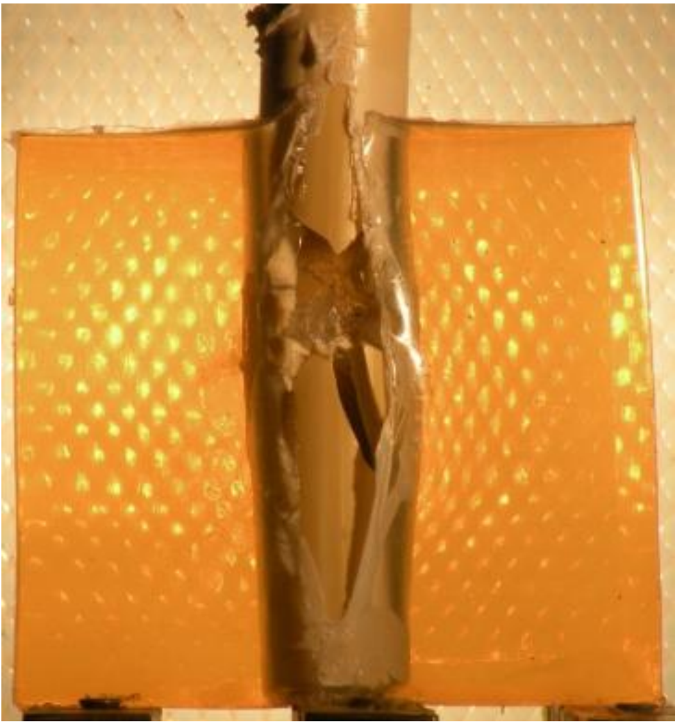
Rear view of femur simulant target shot by 45 Auto JHP. Note complete fracturing of bone.
