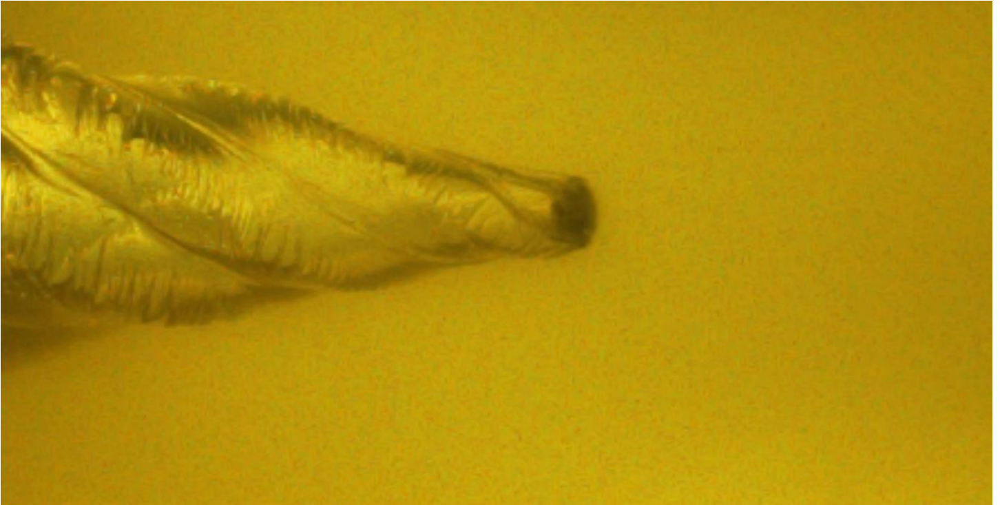
Laminar flow beginning at 9.6" penetration (note gelatin now in contact with side of jacket segments)
