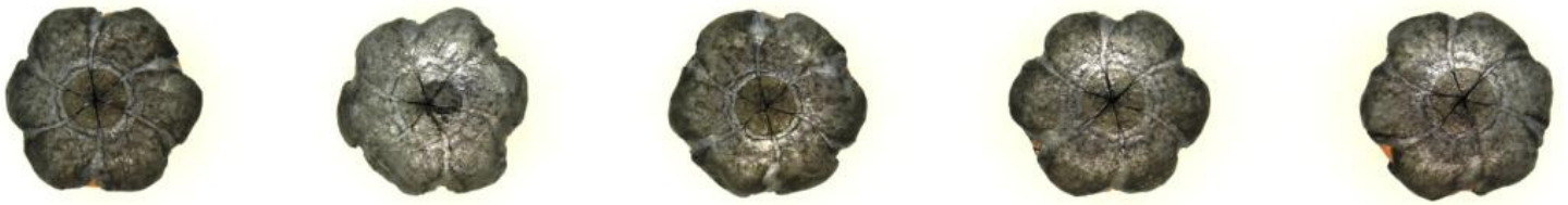
9mm Luger Hornady Critical Defense 115gr through bare gelatin
