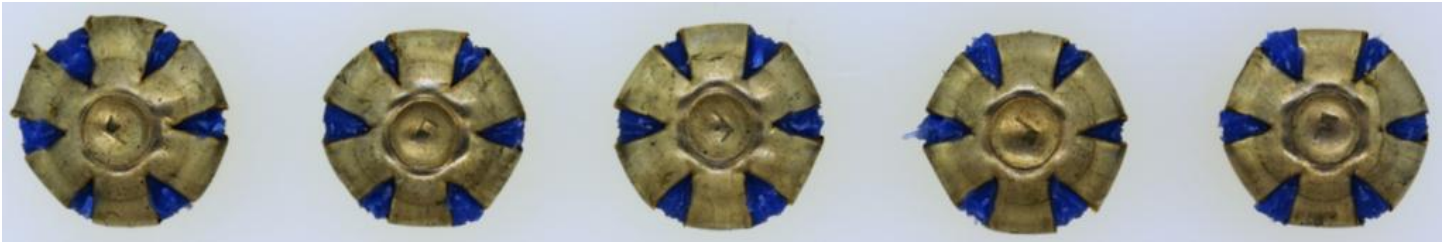
45 Auto Federal Guard Dog EFMJ 165gr through bone plate
