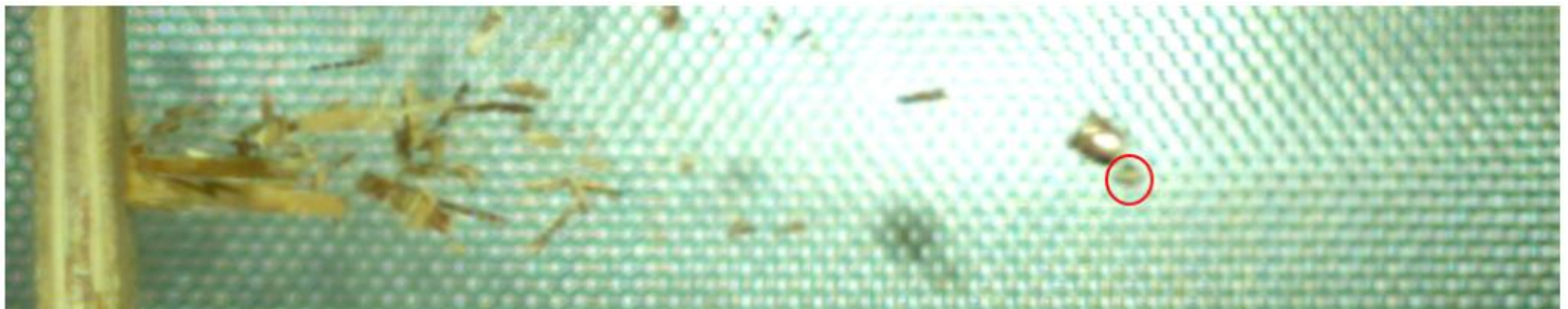
45 Auto 200gr JHP after impact with plywood barrier (plywood plug circled in red)
